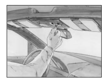
5. Pull the latch handle rearward away from the windshield and hold it until the convertible top is fully lowered.
